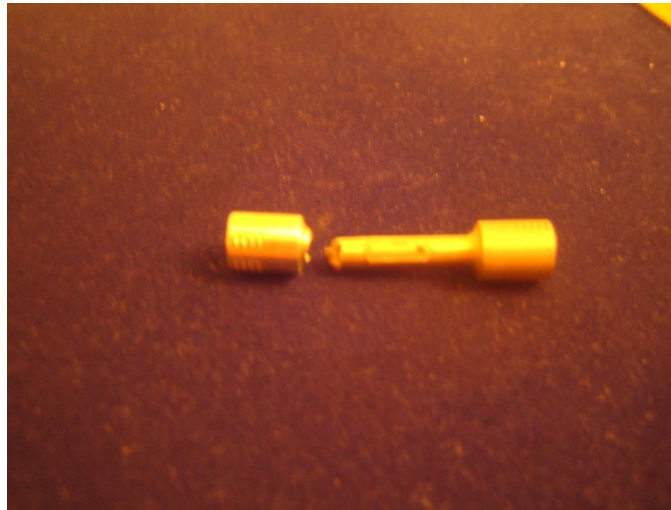
Figure 4. 5 A failed tensile sample
