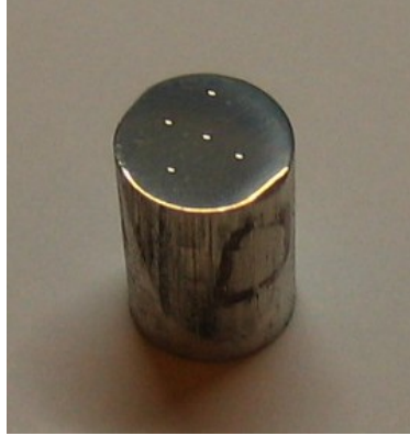
Figure 4. 8 Indentations on an extruded and polished sample
